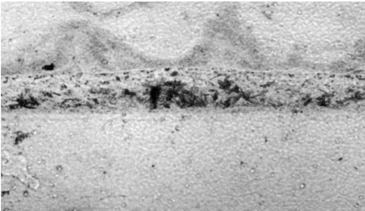
Figure 23. Thin section demonstrating phyllosilicates (gray-black) within macroquartz of horizontally-layered type agate immediately below the border to macroquartz (upper field of micrograph) from inside of a spherulite; locality 4; parallel polars, i.e.f. ca. 0.6 mm.
